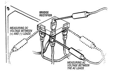
Normal DC voltage running out of the rectifier (in volts DC) is measured across the two DC connections of the bridge rectifier, that is + and - as illustrated.
