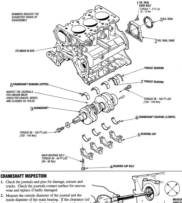
inside diameter of the main bearing. If the clearance (oil clearance) exceeds the limit, replace the main bearing and also the crankshaft, if necessary. Otherwise, fabricate an undersized crankshaft and replace the main bearing with an undersized one. Standard Limit
