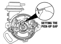
Adjust the point gap of the pick-up assembly between the rotor and the pick-up.
