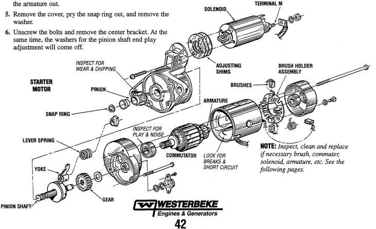
**4.** *Return test:*. With a battery connected to the solenoid terminal M (-) and to the starter body, manually pull out the pinion fully. The pinion must return to its original position when released from holding by hand.
