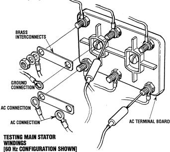
**NOTE:** The studs on the AC terminal board are identified by the six red wire that attach to them. These wires are numbered 1 thru 6. There are no numbers on the terminal block.
