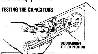
**WARNING:** Capacitors must be discharged before handling as they store electricity and can pack a potentially lethal charge even when disconnected from their power source.
