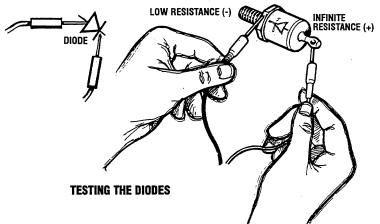
A low resistance should be found with the leads in one direction, and infinite resistance (blocking) in the other direction.
