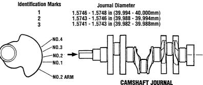
**CRANKSHAFT BEARING THICKNESS**
