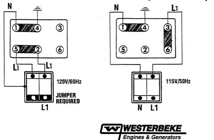
**NOTE:** When changing from 60Hz to 50Hz, make certain the ground wire is properly repositioned according to these diagrams.
