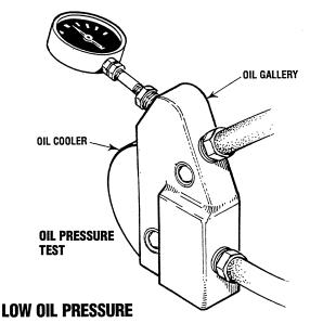
The specified safe minimum oil pressure is 4.3 + 1.4 psi (0.3 + 0.1 kg/cm<sup>2</sup>). A gradual loss of oil pressure usually indicates worn bearings.
