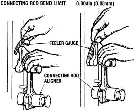
CONNECTING ROD TWIST LIMIT 0.004in (0.1mm) CONNECTING ROD BIG END TO CRANKSHAFT SIDE CLEARANCE Standard 0.0039 - 0.0098in (0.10 - 0.25mm)
