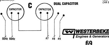
**WARNING:** Capacitors must be discharged before handling as they store electricity and can pack a potentially lethal charge even when disconnected from their power source.
