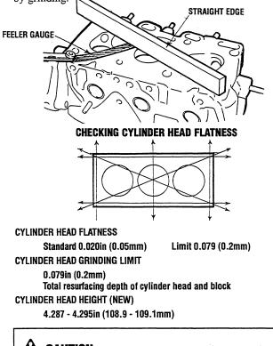
A CAUTION: No more than 0.079in (0.2mm) of stock may be removed from the cylinder head and cylinder block mating surfaces in total.
