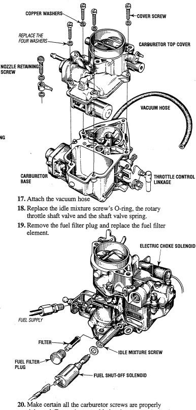
20. Make certain all the carburetor screws are properly tightened. Fasten the assembled carburetor on the intake manifold using new gaskets (use sealant). Replace the two nuts and washers and tighten the carburetor to the manifold.
