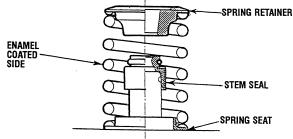
Use the valve spring compressor to compress the valve springs. With the valve spring compressed, remove the retainer locks.
