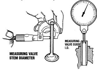
VALVE STEM SEAL TO VALVE GUIDE CLEARANCE
